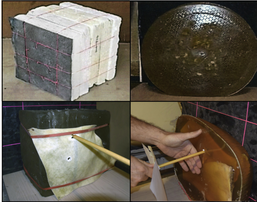
Fig. 4. Foam block (upper left), ballistic gel (upper right), rawhide (lower left), and ballistic gel encased bovine scapula (lower right) targets.
